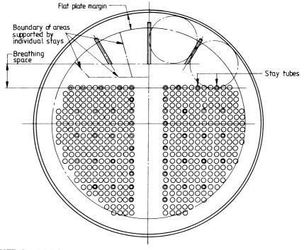
NOTE. See **4.1.2** for methods of attachment of end plates to shell. (b) Boiler with directly welded end plate
