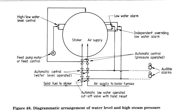
Figure 48. Diagrammatic arrangement of water level and high steam pressure automatic controls and cut-outs for boilers fired with solid fuel complying with section six
