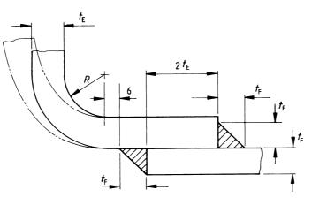
NOTE. The furnace to end plate attachment is suitable for front ends only, or in cases where there is no impingement of flame or hot gases. (b)
