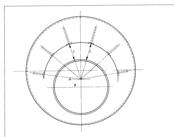
NOTE. The distance A - B between the centre of the stay circle and centre of furnace is not to be less than 3t + 63, where t is the thickness of the end plate (in mm). (c) Typical arrangement of end plates on a single furnace boiler
