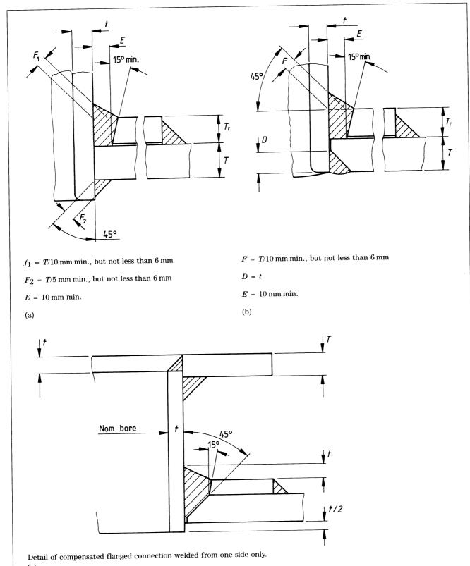
(c) NOTE. Where a single side weld is used, the technique and electrodes used are to be demonstrated to the inspecting authority on separately prepared test specimens to prove full penetration with sound weld metal at the root.
