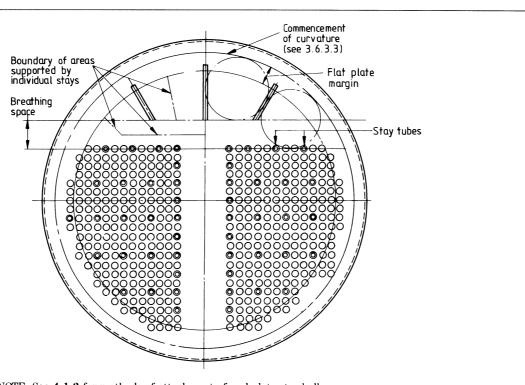
NOTE. See **4.1.2** for methods of attachment of end plates to shell. (a) Boiler with flanged end plate
