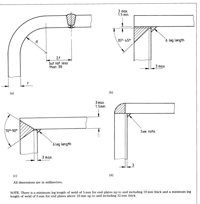
Figure 31. Attachment of end plates to reversal chamber or firebox wrapper plates
